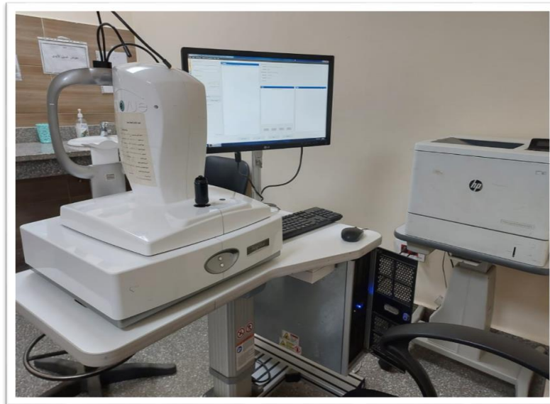
Figure 1: Anterior Segment Optical Coherence Tomography used in this study.
